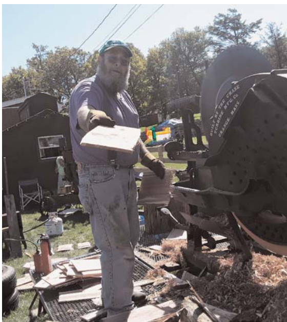
This Chase Turbine custom rip saw for making shingles – Mfg. Co, Orange Mass, patented Feb 19, 1889 by Chase Turbine Mfg. Co., Orange, Mass.
