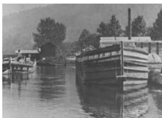
: This unique scene clearly shows the difference between a light and loaded boat. The boat on the right is a light, or empty boat, it is floating high on the water. The boat on the left is loaded down with cargo and sits lower in the water. Behind the light boat is the George Hoar Sand Mill. The large masonry chimney of the Ellenville Canning Factory can be clearly seen, and in the center of the photograph is the D&H Canal office.
